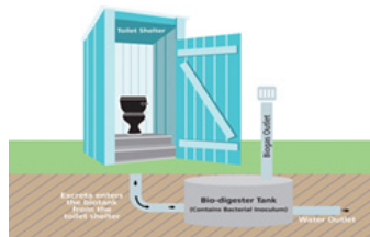
Figure 1.13: Schematic view of toilet linked biogas plant
