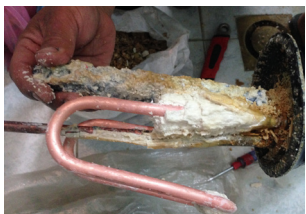
Figure 1.7: Boiler heater with 'Scale'
