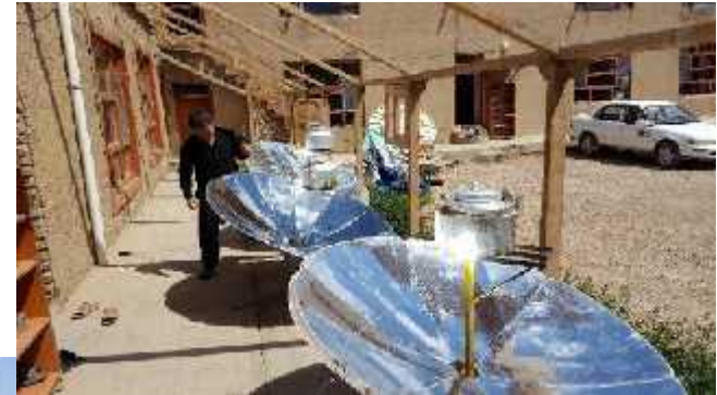
Solar Cooker with mirrors
