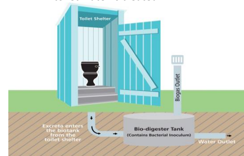
Picture. 1 Schematic view of Toilet linked Biogas Plants (Courtesy of Wockhardt Foundation)
