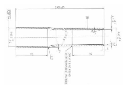
**Type of Pipe**: uPVC non-pressure pipe 4-inch diameter
