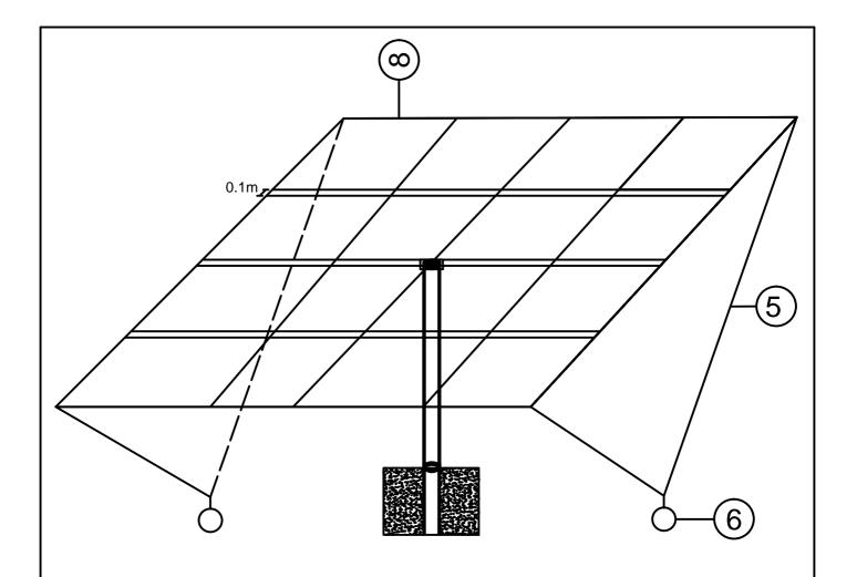
5-Angle located which is connect to the Wheel 4NO deferent length Square shape profile having (40\*40)mm size 3mm thickness 5kg weight per m
